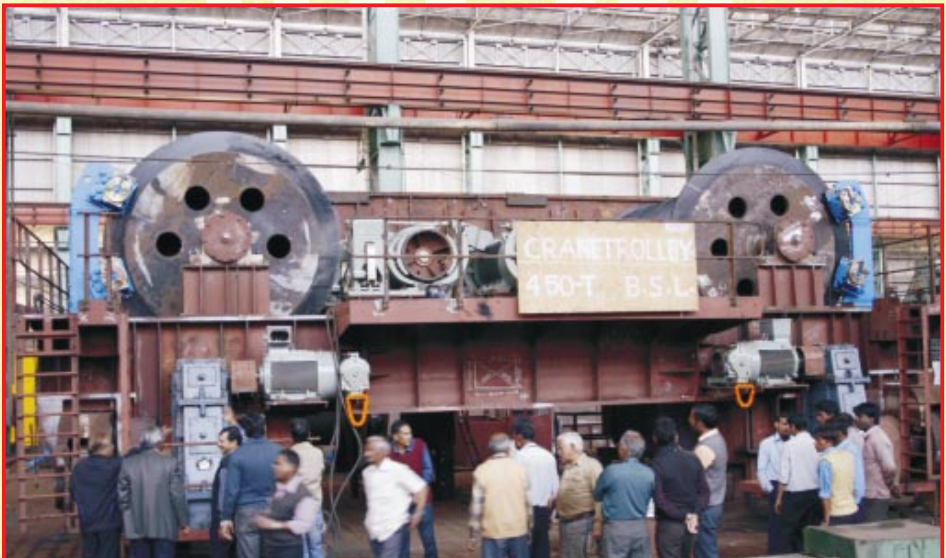
Assembly of 450 Ton EOT Crane trolley before despatch
