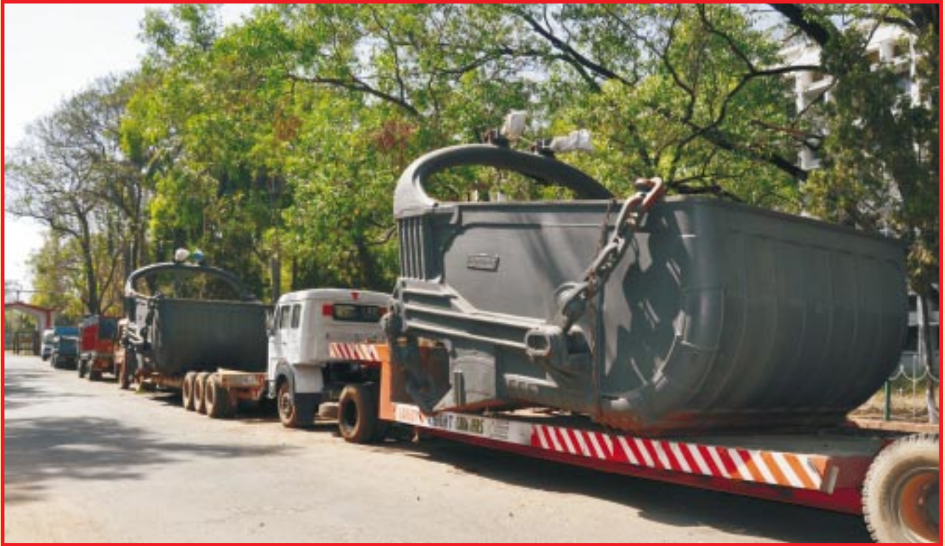
Dispatch to NCL of bucket of capacity 24 cum for Dragline
