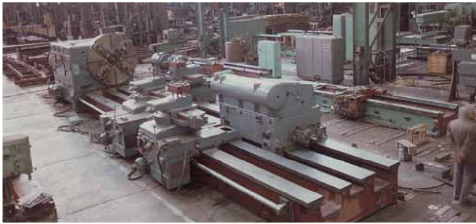
4 - Guideways CNC Roll Turning Lathe Model : LRT 160N/8M Swing over bed - 1600 mm
