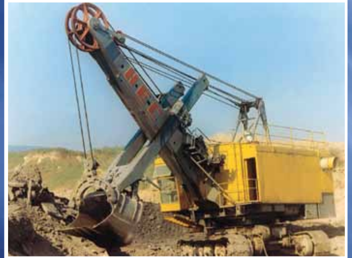
Electric Rope Shovel, 5 Cu. M.
