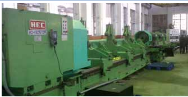
CNC Deep Hole Boring Machine model BDH 140N/12M with bottle boring facility (Customer : O.F. Kanpur)
