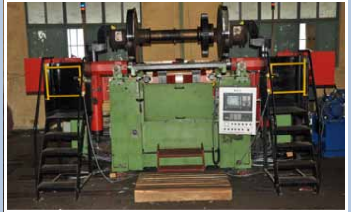
CNC Under floor wheel lathe
