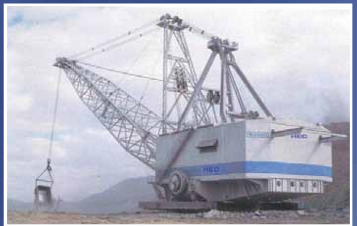
Dragline, 24cum Bucket capacity, 96m Boom length
